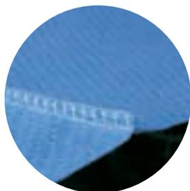
A **SERGED SEAM** is a basic stitched seam that's appropriate for exposure to non-hazardous substances. Overlap stitching provides strength and durability.
