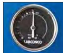
Monitors pressures between 0 and -29 inches of mercury. Mounts atop the glove box. Includes vacuum gauge, hose, mounting bracket and fittings. **Requires installation and 0.562" diameter hole.** Included with Precise Controlled Atmosphere Glove Boxes. Shipping weight 2 lbs. (0.9 kg)
