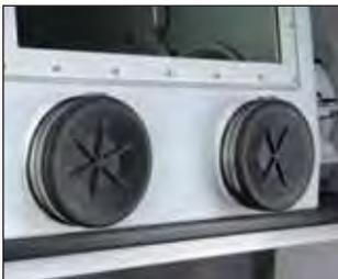
May be placed over glove ports with or without gloves attached to facilitate evacuate/fill operations and preserve inert atmosphere. Molded rubber. Includes two clamps. Set of two. Shipping weight 3.5 lbs. (1.6 kg)
