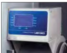
For automatic control of the main chamber pressure (-5 to +5 inches of water gauge), main chamber purging and filling cycles (up to 199 cycles), and transfer chamber evacuation and filling cycles (up to 199 cycles). Regulate vacuum/pressure between -5 and +5 inches of water gauge in the main chamber
