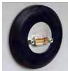
Provides a leak-tight connection for data transfer to a customer-supplied printer or computer located outside the glove box. Includes sealed 9 pin connector (D-subminiature with male pins on one side and female pins on the other) and 10' cord. **Requires installation and drill hole.** Installation Kit 5241100 is recommended. Shipping weight 1 lb. (0.5 kg)
