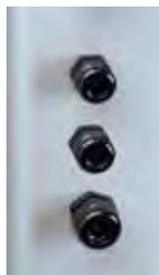
Provides three pass-through ports with sealing ID ranges 0.230/0.395, 0.230/0.530 and 0.450/0.705, useful for sealing cords and plumbing. **Requires installation and drill holes.** Installation Kit 5240800, with drill bits, is recommended. Shipping weight 0.5 lb. (0.2 kg)
