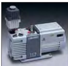
For evacuating the main chamber and/or transfer chamber. Ultimate vacuum (total pressure) is  $2 \times 10^{-3}$  mBar (1.5 micron). Consist of on/off switch; two inlet adapters (1/2" and 3/4" OD); mode selector with High Vacuum and High Throughput positions; and gas ballast with closed, low flow and high flow positions. Single phase, direct drive motor, totally enclosed and fan cooled.
