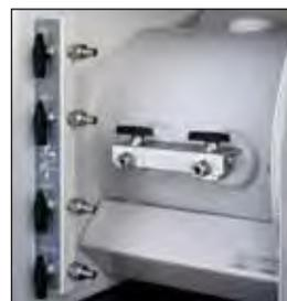
Includes six each manual ball valves, pressure relief valve, compression fittings, hose connector fittings, holesaws, O-rings and nuts to add four service valves to the main chamber and two service valves to the transfer chamber. Two of the valves on the main chamber and two on the transfer chamber may be used for evacuating and filling. The remaining two on the main chamber are for drying train connections.
