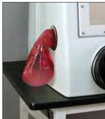
Provides a 4.5" (11.4 cm) diameter pass-through port to attach an external waste bag. Rubber stopper plug is provided to close off the port from the inside of the glove box. Minimum waste bag size is 8.5" wide.
