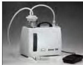
Evacuate fluid spills in the glove box interior. Chemical-resistant diaphragm pump draws 12 liters/minute with on/off switch and manual/foot pedal control switch. Autoclavable, two-liter glass container allows safe collection and disposal of hazardous liquids. Float valve automatically
